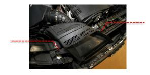
3 Disconnect the air flow sensor. Loosen the 2 x hose clamps on the airbox and turbo inlet pipe.
