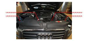
Premove the air intake duct by unscrewing the 2 x T25 bolts.
