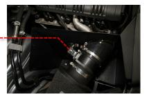
15 Check that all hose clamps are tight and that everything is attached correctly. Test drive the vehicle to ensure vehicle performs correctly and there are no leaks/part interference during operation. Your installation is now complete!
