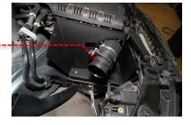
12 Install the Revo air filter onto the air flow sensor unit and secure with the 70-90 hose clamp.
