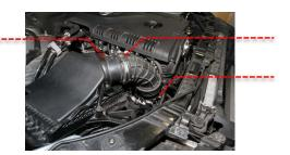
4 Remove the complete airbox assembly by pulling up on the main housing so it pops off the rubber mounting points.
