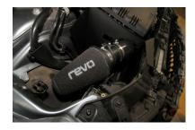
Reinstall the front air duct, once installed push the top section of the heatshield into the tabs at the top to hold it in place, as shown.
